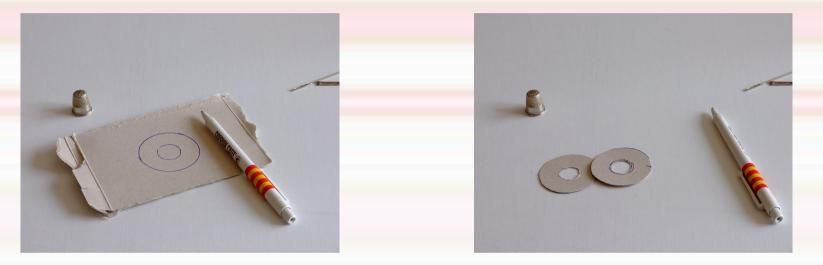
Placing the 2 pieces of carton, one on top of the other with the template drawings uppermost, cut around the circles as seen here, above right
